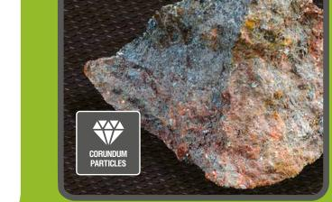
Unique film containing corundum particles provides exceptional anti-slip properties and wear-resistance.
