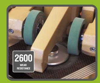
The highest level of resistance to surface wear (not less than 2600 rotations, Taber test according to EN 438-2:2016)\*.
