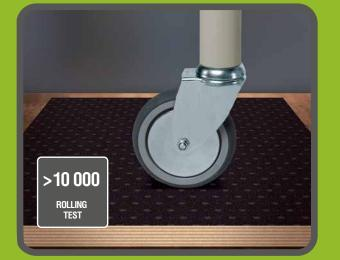
SVEZA Titan is resistant to loading of roller wheels (more than 10 000 cycles, rolling test according to standard SFS 3939).
